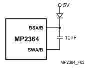
Figure 2—External Bootstrap Diode
