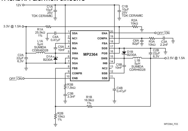
Figure 3—2.5V @ 1.5A and 3.3V @ 1.5A Application Circuit
